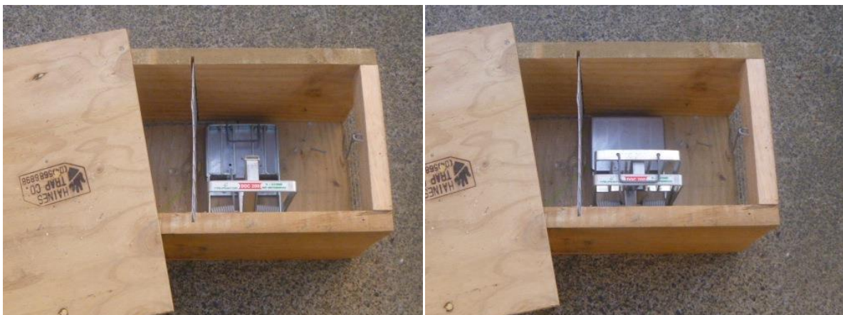
Figure 1: Doc 200 Trap Safe (Left) and Set (Right)
